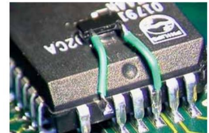
Figure 4 Chip component soldered to surface mount component using jumper wires. Note: One lead of surface mount component is shown lifted.
